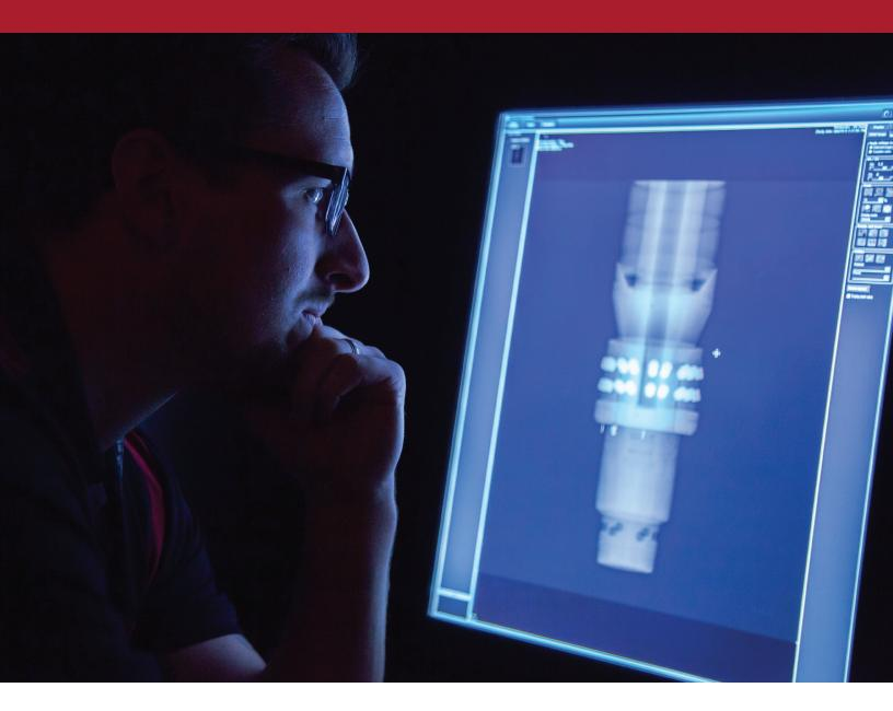
What is NDT? Nondestructive testing is the examination of an object or material without affecting its future usefulness. Nondestructive tests are performed to identify internal or external imperfections; to determine structure, composition, or properties; or to measure geometric characteristics - without affecting the form, fit, or function of the test object.
